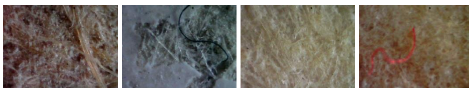
Figure (12), shows the fibers characteristics of secondary support and some impurities between the fibers
