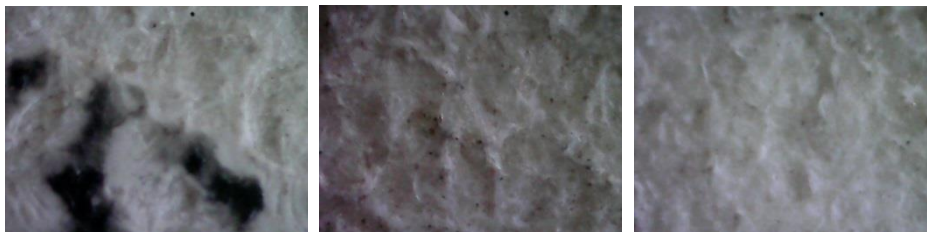
Figure (10), shows the surface characteristics of primary support and some silver grains distribution in scratched part of the image.
